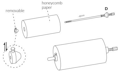
As shown in figure, slide removable piece off of the bar, thread bar through the honeycomb paper and return removable piece.
