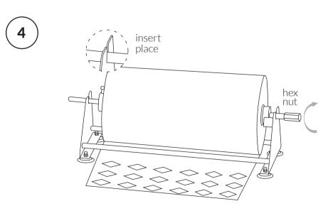
As shown in the figure, place fixed honeycomb paper on A and B, and rotate the hexagonal nut to adjust the resistance.
