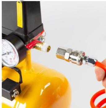
Remove the quick release female fitting from airline and screw onto output on right hand side of compressor. Tighten with a spanner. Do not overtighten.
