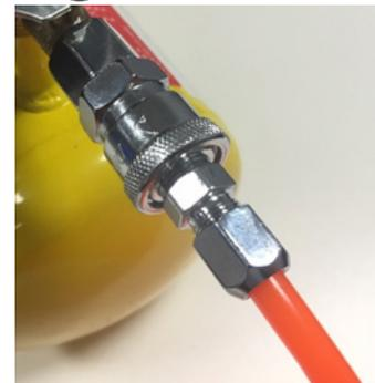
Insert male quick release fitting on the end of the airline into the female fitting in step 4.
