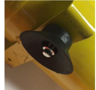
Fit the four rubber feet with four bolts/nuts and tighten with a spanner/socket
