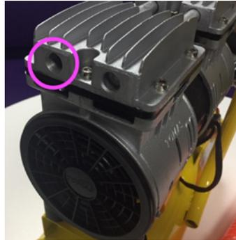
Locate the threaded hole. Top left hand side of the compressor
