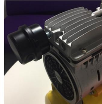
Screw the air filter into this threaded hole and tighten by hand only
