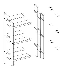
Move the assembled frame into position in your store and then tighten all the screws. This will allow the unit to sit more squarely on slightly uneven floors.
